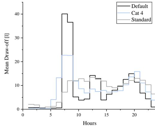
**Figure 2.** Mean hourly draw-off profiles of the created 3 different 60 min load profiles (Default, 4 Categories option from Jordan and Vajen (2001) and load profile created from standard EN 12831-3).
