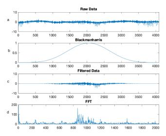
Figure 4. Acoustic chemometrics signal processing steps.
