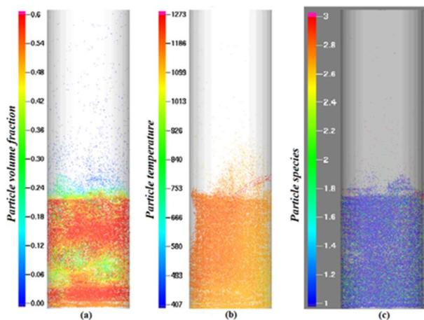
**Figure 3.** (a) Bubbling fluidization, (b) temperature of bed particles, (c) distribution of particle species
