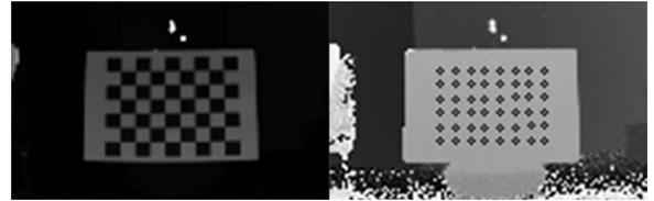
**Figure 5:** Left: The amplitude image of SwissRanger 4000. Right: Detected corners that are localized in the depth image.
