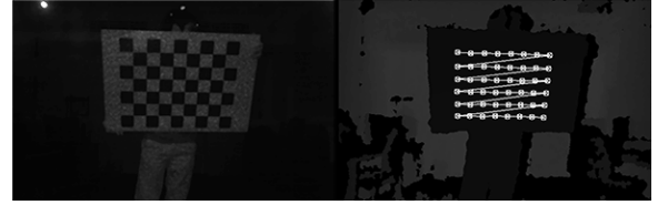
Figure 4: Left: The blurred IR image of Kinect camera. Right: Detected corners that are localized in the depth image.
