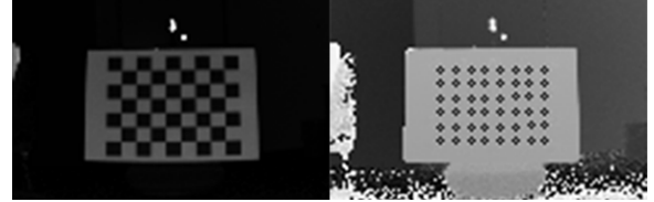
Figure 5: Left: The amplitude image of SwissRanger 4000. Right: Detected corners that are localized in the depth image.
