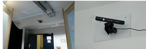
Figure 4: The Kinect sensor mounted on the rear end of the CAVE.
