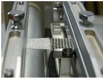
Fig. 3-1 Peeling Strength Test Using KES FB1 Tensile Tester
