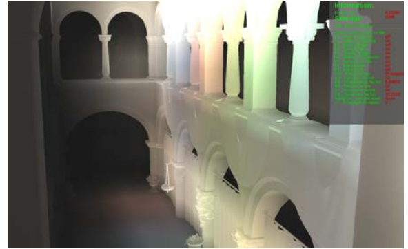
Figure 5: The sponza scene rendered using only indirect illumination and without any diffuse texturing. Note that the indirect lighting has been slightly exaggerated in this image.
