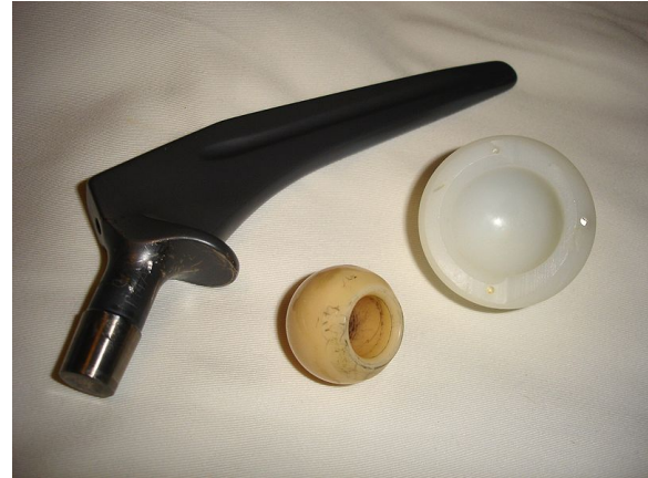
Figure 3: Photograph of a titanium stem, a ceramic head and a polyethylene acetabular cup.
