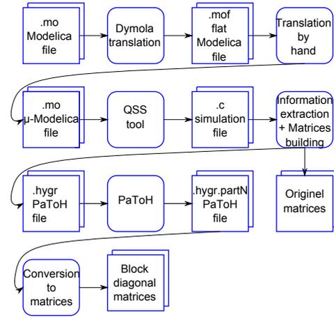
**Figure 10.** Software tool-chain
