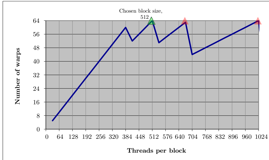
Figure 5: Impact of varying block sizes on multiprocessor occupancy.
