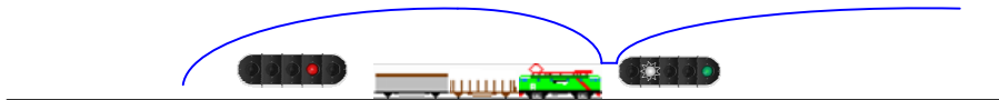
Figure 3: The first train has left the block section which makes the signal green, but the following train gets no update of the signal aspect and has to slow down to surveillance speed (blue curve).
