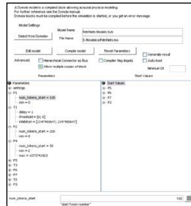
Figure 11: Parameter dialog of the DymolaBlock in Simulink
