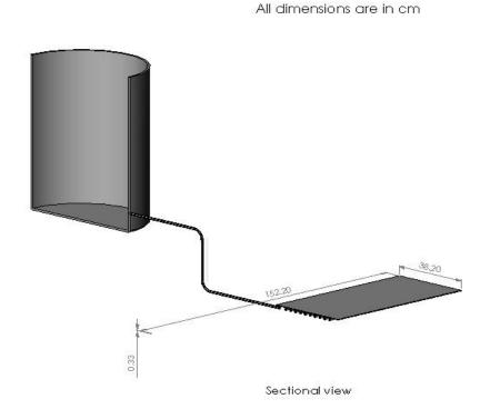
Fig. 2 Sectional view of the radiator assembly
