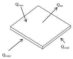
Fig. 3 An energy balance on the nocturnal radiator.
