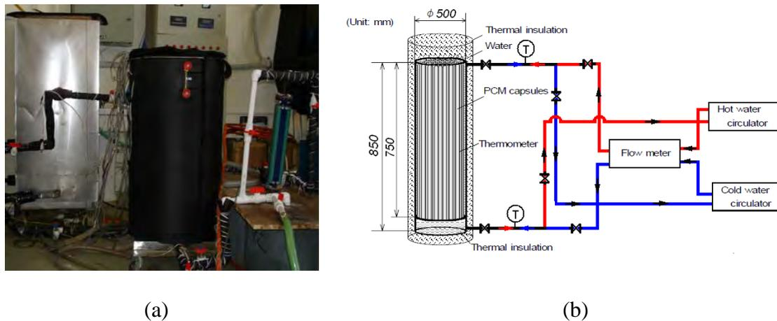
Fig. 1 Experimental setup (a) Photographic view (b) Schematic of LTES system
