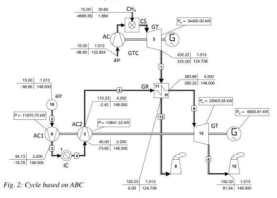
As shown in Fig. 2, the air bottoming cycle without solar energy was examined. The C-ABC had the same characteristics as the S-ABC, except that the optimum pressure ration was 2.17 and 1.91, respectively. Also the air mass flow was fixed at 148 kg/s.
