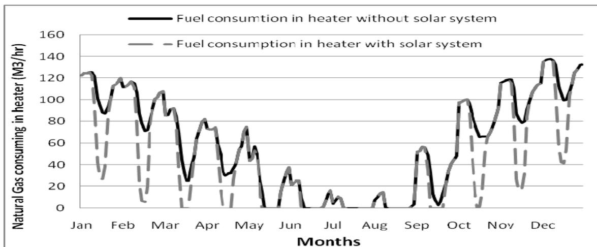
Fig. 6. The heater fuel (natural gas) consumption required for preheating gas in 2009
