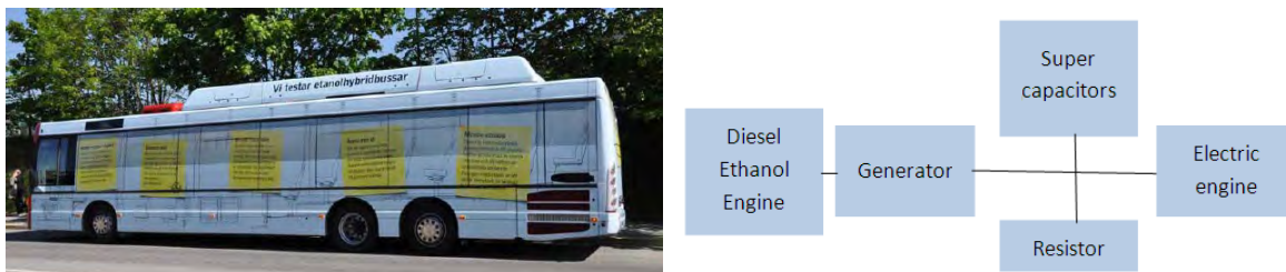
Fig 1. The Scania OmniLink ethanol hybrid bus and a schematic illustration of the series hybrid powertrain [Photo: Stefan Wallin, SL]
