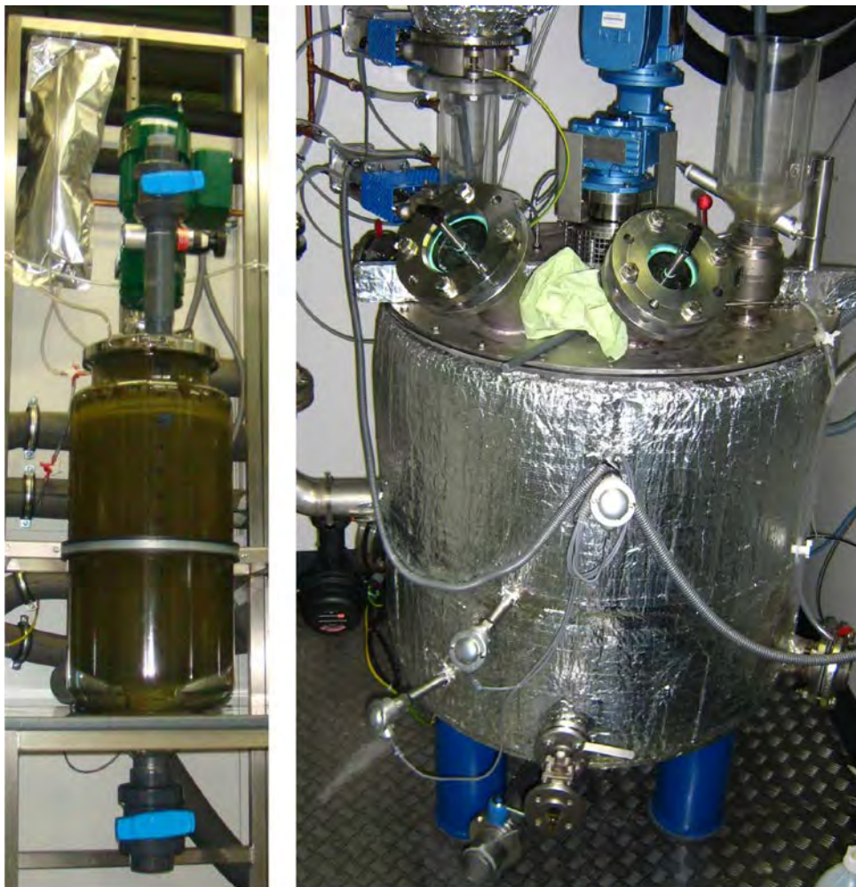
Fig. 1. Left: One of the three continuous 22 l digesters; Right: continuous 390 l digester.
