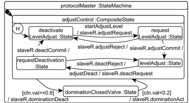
Figure 2. Protocol Behavior of the Master Controller
