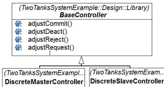
Figure 7. Message Definition of the Controller Classes
