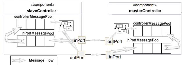
Figure 8. Internal Message Pool Representation and Message Flow
