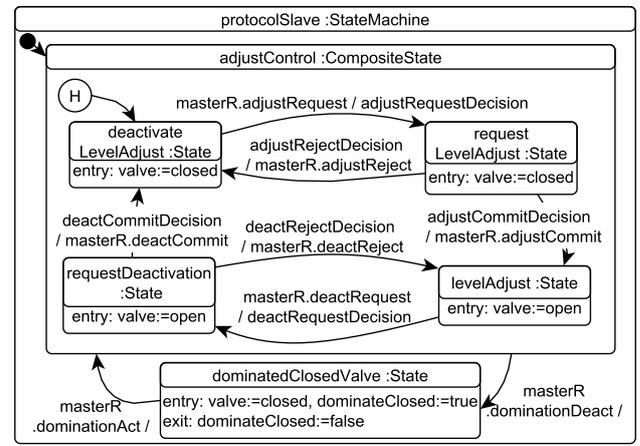
Figure 3. Protocol Behavior of the Slave Controller
