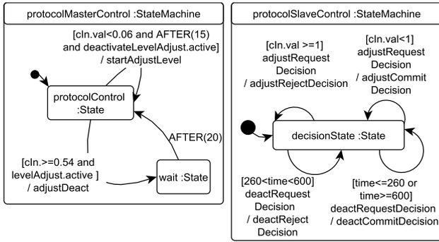
Figure 4. Protocol Control Behavior of the Controllers
