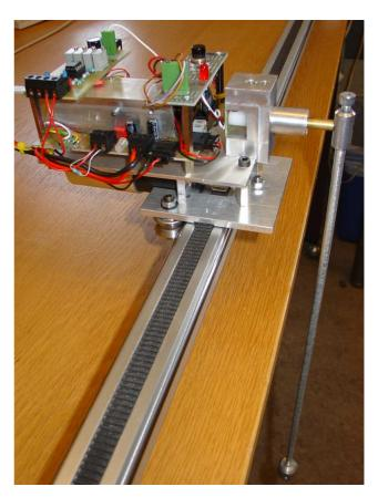
Figure 3: Photo of the cart and pendulum system described in Section 3.
