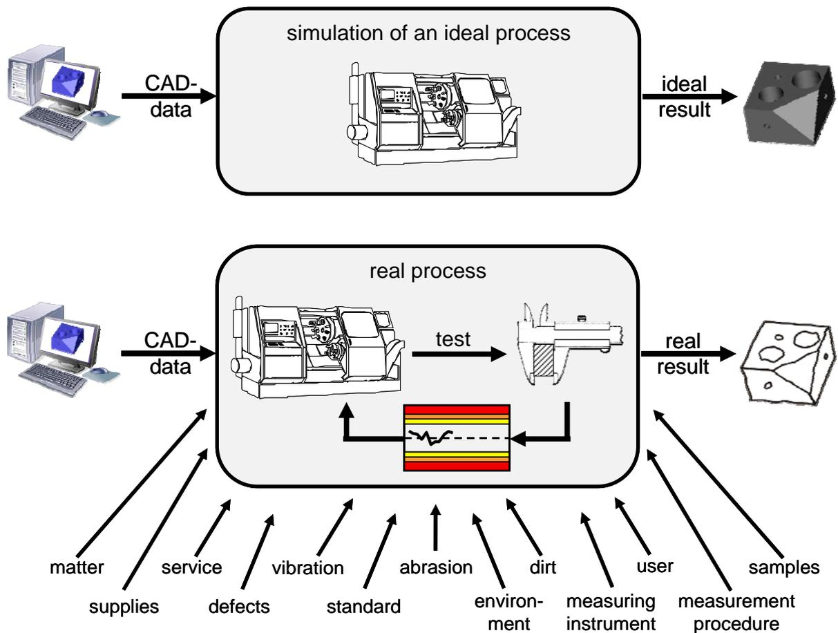
**Figure 1:** Difference between a simulation model and reality
