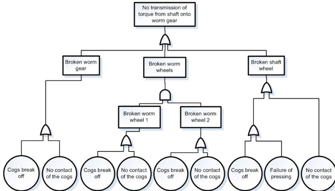
Figure 3: Fault Tree for the gearbox of a motor drive (cf. Zacher, 2006)
