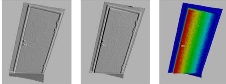
Figure 1: Reconstructed surfaces from two scans of the same door and exaggerated, color coded difference.
