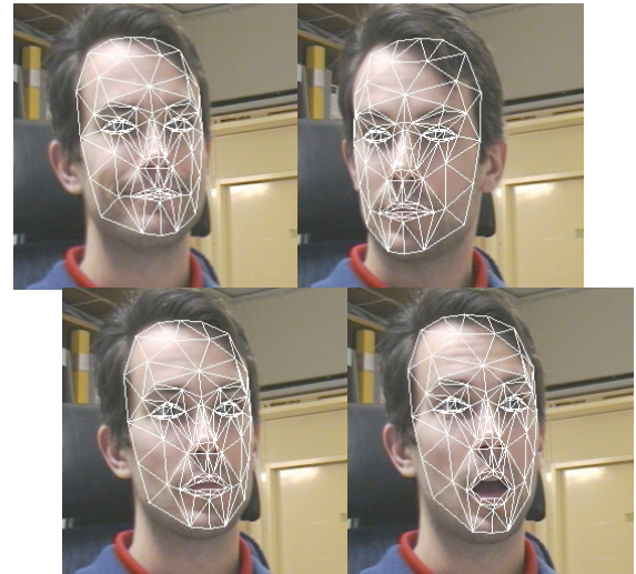
Figure 4: Automatic face and facial feature tracking. The simple face model adapts to each frame in the sequence (every tenth frame shown), and MPEG-4 FAPs can then be extracted from the model.
