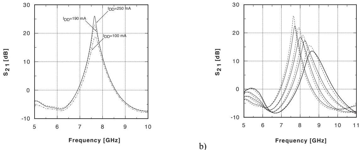
Fig. 3. Measured  $S_{21}$  a) at state 000 for different values of  $I_{DD}$  b) at all eight center frequency tuning states (i.e. 000-111) when  $I_{DD}=250\text{mA}$ .
