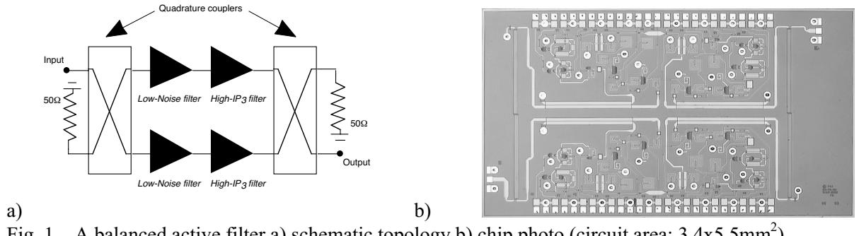
Fig. 1. A balanced active filter a) schematic topology b) chip photo (circuit area:  $3.4 \times 5.5\text{mm}^2$ ).
