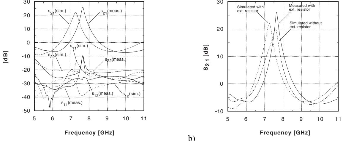
Fig. 2. Measured and simulated small signal data at state 000 a) s-parameters b) transmission gain  $S_{21}$ .
