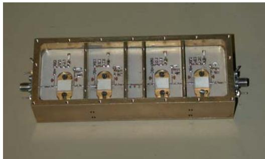
**Figure 4** The amplifiers microwave circuits.
