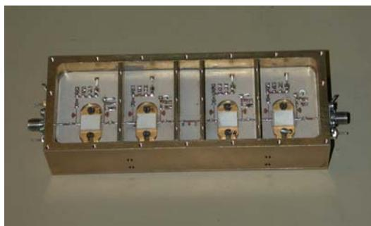
**Figure 4** The amplifiers microwave circuits.
